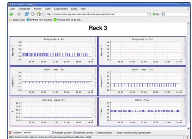
Figure 2: Web interface of our monitoring displaying sensor information of rack three.
